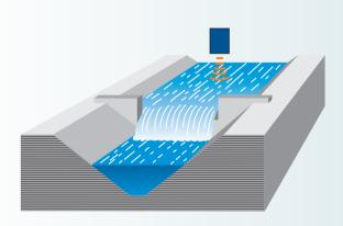
Nivo Ultrasonic Level Transmitter provides trouble free sensing of
