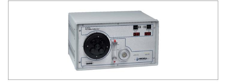
The S904 is a completely stand-alone and transportable calibrator for humidity sensors, requiring no external services other than mains power. The calibration chamber features 5 interchangeable ports to accommodate virtually any brand, type or model of sensor. This calibrator is ideal for companies or organizations looking to calibrate large numbers of probes in a laboratory or field setting.
