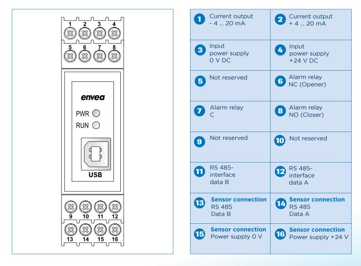
If desired, the Dusty can be combined with a converter. This converter converts the measuring signal into a continuous 4 ... 20 mA signal. This provides the operator with a trend signal from which any limit value can be derived. For very large channel diameters you can connect up to 3 Dustys with one converter to improve the trend signal.
